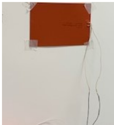
(b) Photograph of measured wall and simulated defect.
