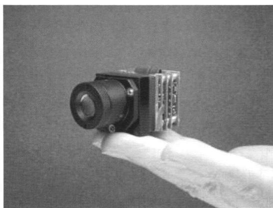
Fig. 9 Proto type infrared imaging camera module designed for 12 \mu\text{m} -640×480 uncooled infrared detector.
