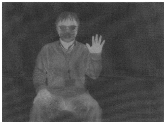
Fig. 8 Infrared image taken by 12 \mu\text{m} -640×480 uncooled infrared detector.
