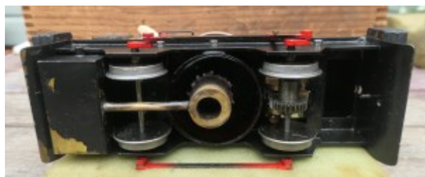
Original meths tank with the replacement annular burner.
