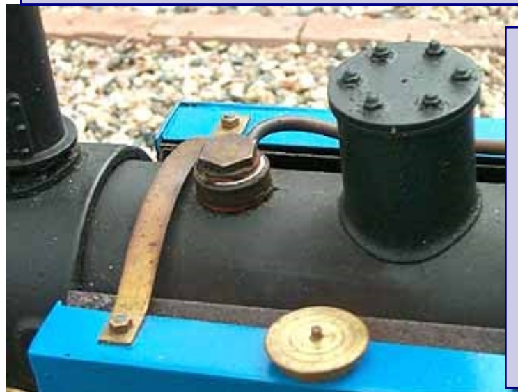
A closeup of the harness assembly attaching the trailer to the locomotive.
