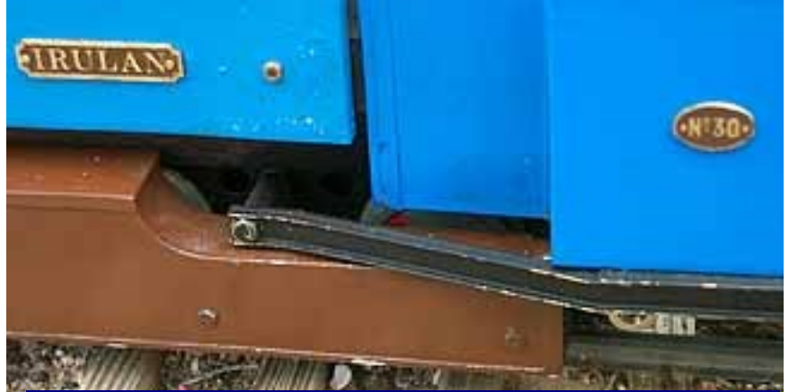
A closeup of the harness assembly attaching the trailer to the locomotive.
