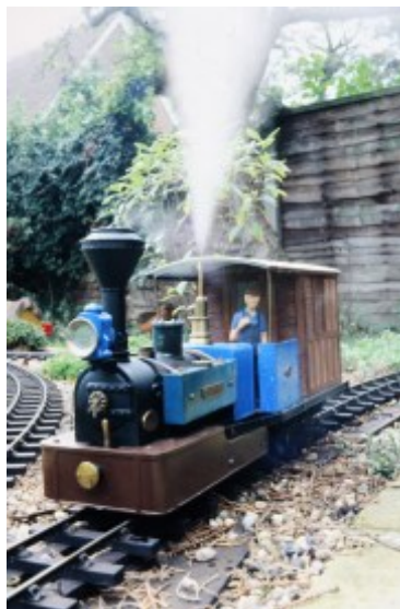
Irulan turning a corner, showing its articulation
