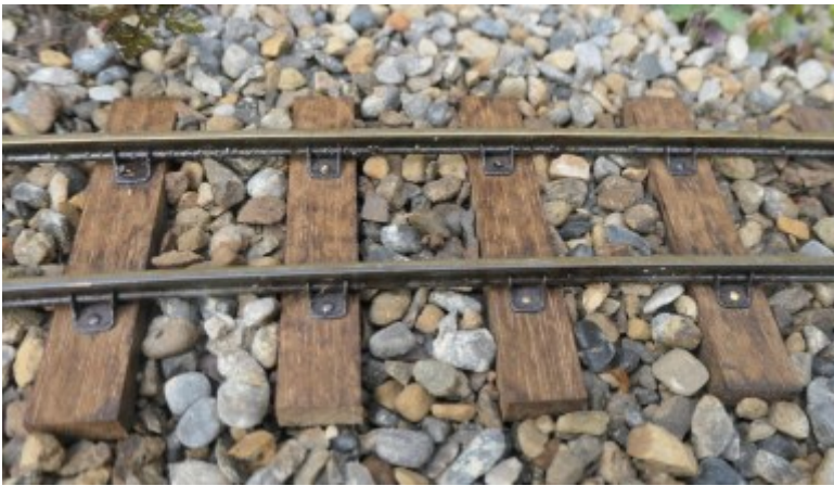
Bassett Lowke pre-WW2 rail and chairs on new sleepers in 2024
