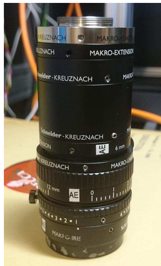
Figure 3.4: A photo of the Schneider Optics camera lens kit used for the 78 rpm discs.
