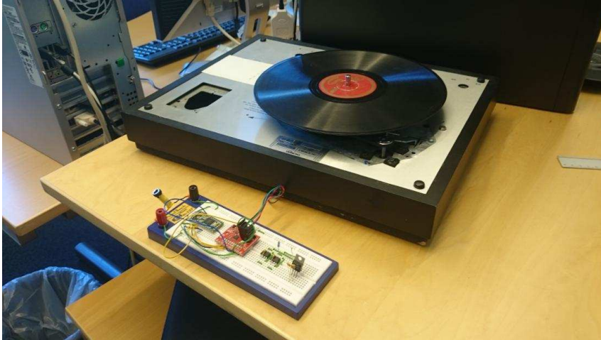
Figure 3.7: A photo of the Arduino Teensy connected turntable provided by SICK IVP.
