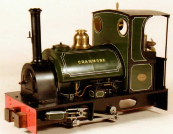
This exquisite Cranmore Peckett was made by David Hick one of the finest builders of 16mm-scale locomotives. Like the prototype, the model has Stephenson's valve gear.
