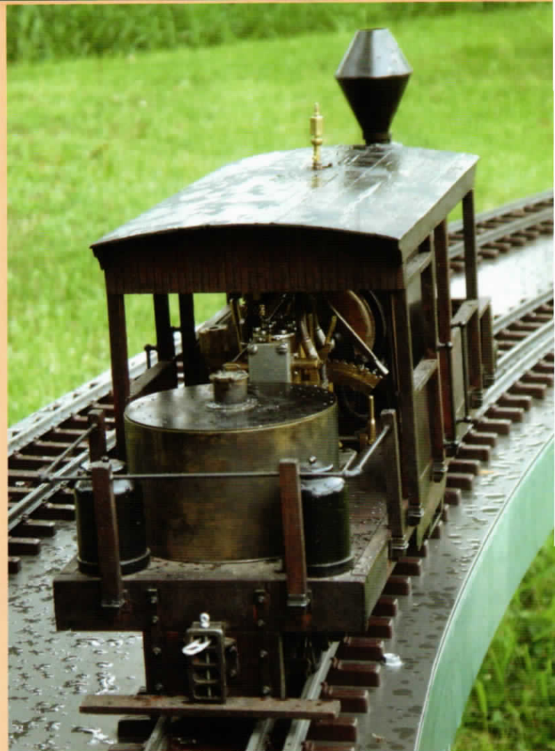
The water tank hides the butane tank. Lots of Trakside Details and Ozark Miniatures parts were used.
