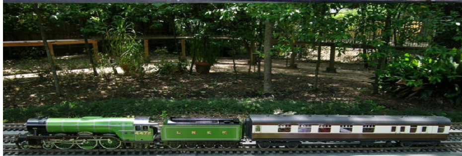
Dave Young's Flying Scotsman (a coal fired conversion by John Shawe) at Steve Speck's Steam Up in Houston, TX. The passenger car built by Peter Comley is based on the prototype pulled by the Flying Scotsman during its US tour. Photo by Arthur Gibson.
