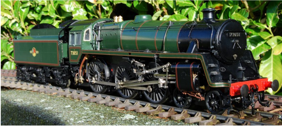
British Railways Standard Class 5 Mixed Traffic 4-6-0 with tender
