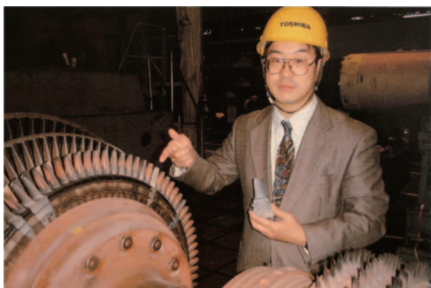
Fig. 14 TMS-82+ and TMS-75 were tested successfully in a 15MW power generation gas turbine.
