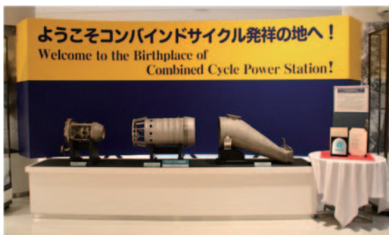
Fig. 2 Premixed Combustor of Higashi-Niigata Thermal Power Station Unit No.3 Series (Essential Historical Materials for Science and Technology.)
