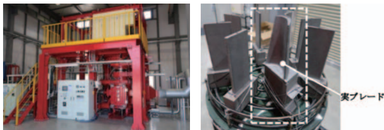
Fig. 25 Developed two-chamber large vacuum heat treatment furnace for ultra-high temperature use, equipped with rapid cooling mechanism by high-speed argon gas flow.
