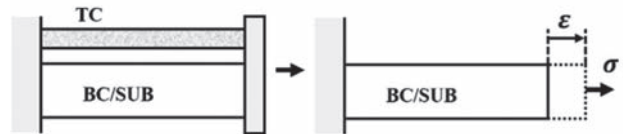
Fig. 4 Mechanistic model for TBC system
