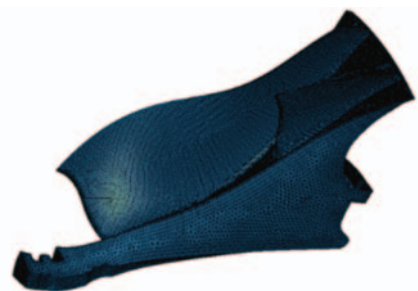
Fig. 4 Structural analysis mesh
