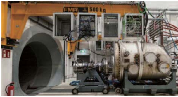
Fig. 9 Combustion Test Rig of Clean Energy Center (9)
