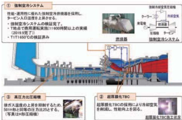
Fig. 4 Design Features of M501JAC gas turbine.
