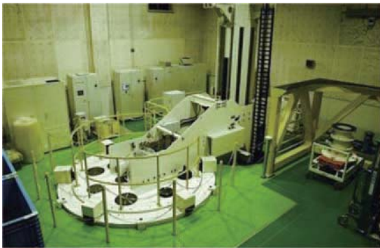
Fig. 8 Engine spin test equipment of ASRC
