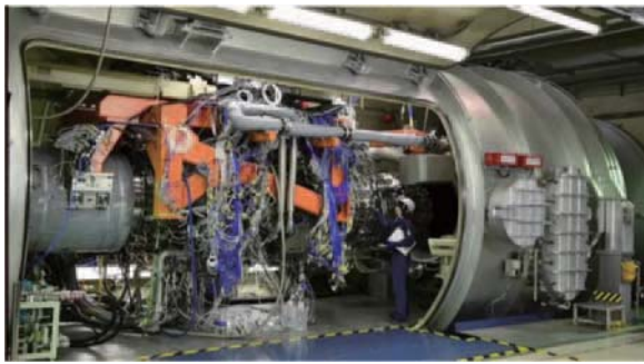
Fig. 16 Altitude test for XF9 at CTC ATF
