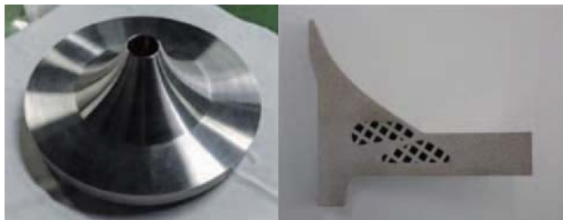
Fig. 19 Test disk and cross section by AM
