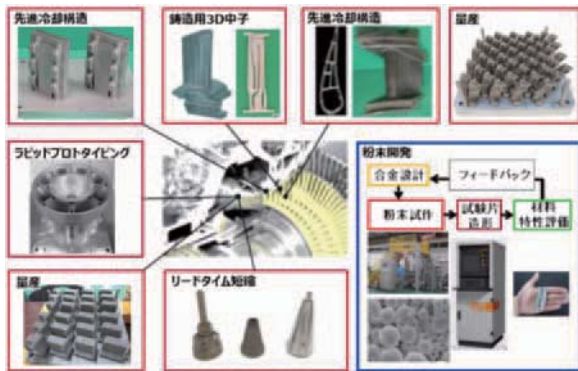
Fig. 10 Examples of AM manufacturing for Industrial gas turbines (Combustor/Turbine)
