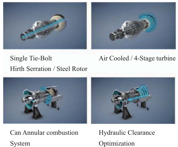
Fig. 3 Common Siemens Energy H- and HL-class design features (7)
