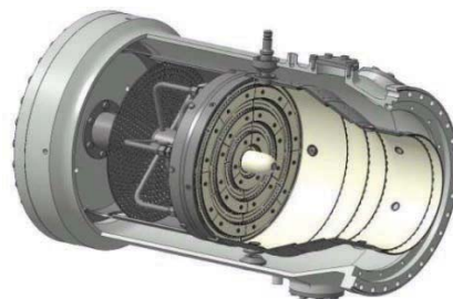
Fig. 6 Dry low NOx combustor with hydrogen combustion
