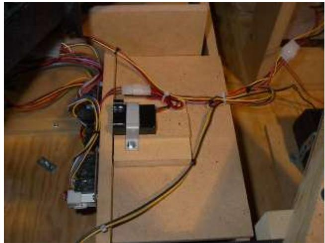
Re-connect the harnesses as required. The connectors on all harnesses will fit only their respective slot in the proper orientation.
