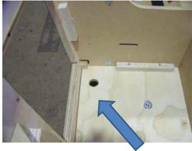
Following the pictures below, please note the placement of the template in the bottom of the table. Using a 2" hole saw and the hole as a guide, bore a 2" hole into the bottom of the table
