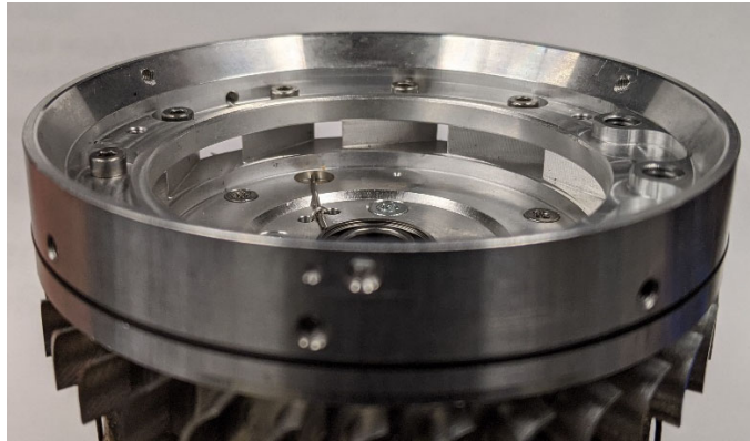
Figure 64. View of compressor radial stator vanes
