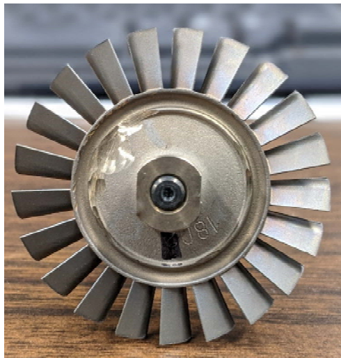
Figure 72. Rear view of turbine rotor
