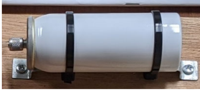
Figure 13. Starting gas tank
