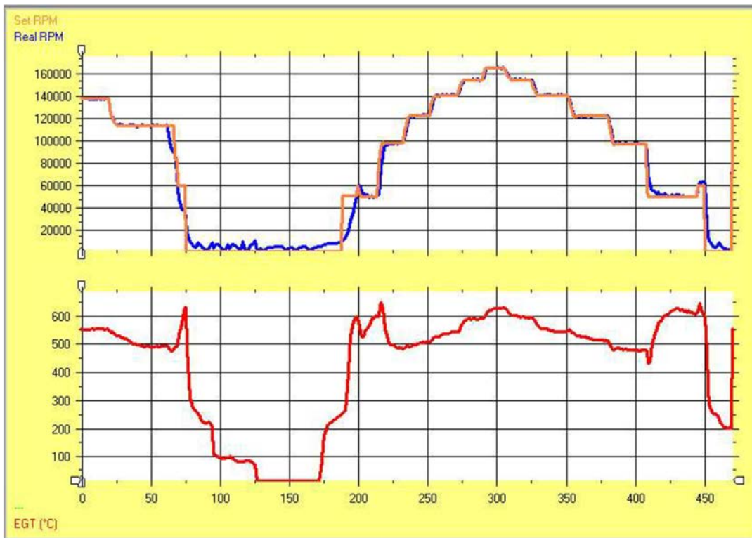
Figure 49. RPM/Set RPM and EGT vs. time Jet-tronic plots – kerosene test run #3
