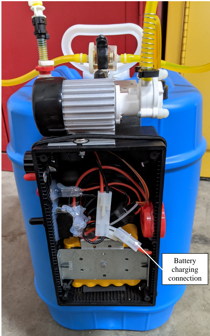
Figure 94. Internal view of mixing container control box
