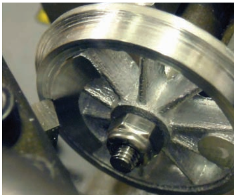
Photo 3c: A wheel is machined on the lathe.
