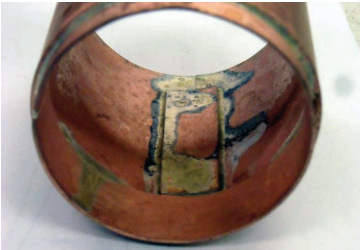
Photo 10: Using Kozo's method the boiler tubes are soldered with a strip over the seam.
