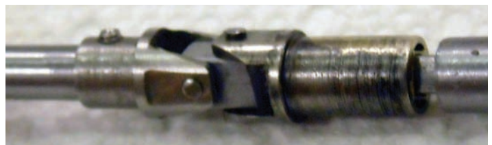
Photo 9: Drive shaft universal joints are turned from 303 stainless; slip joint on lower right is square tool steel. The female end is K&S square stock silver soldered into a hole drilled in yoke.
