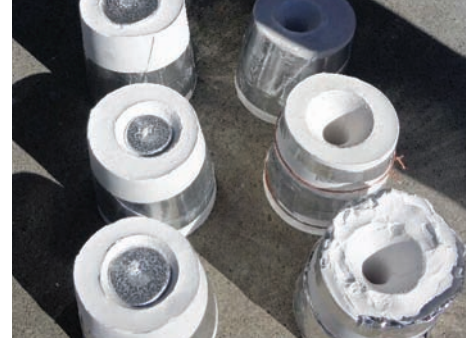
Photo 3b: Wheels are poured with a large sprue which forces the metal into the small crevices.
