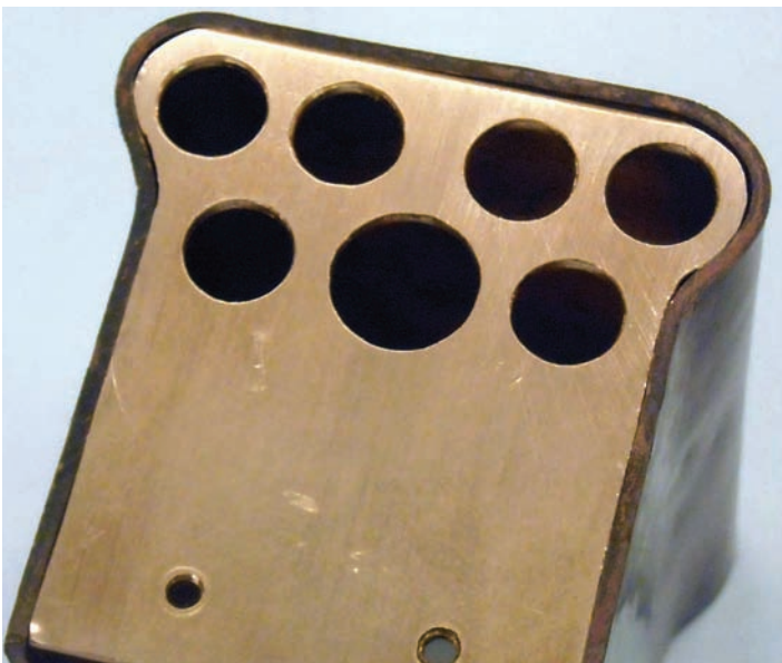
Photo 12: Fire box shape is patterned after 70-ton prototype. Sharp bends were made by cutting a hardwood former and hammering the shell to fit.
