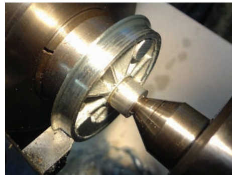
Photo 3d: A tread-cutting tool is ground to shape with a cut off tool (Dremel).
