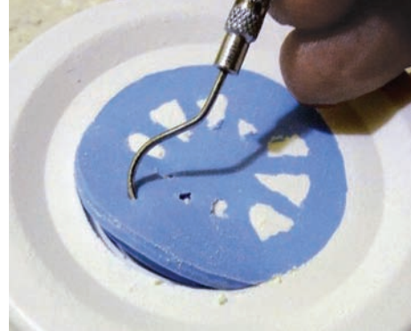
Photo 3a: Silicone positive is removed from Hydrocal mold.
