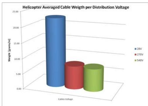
Fig. 8 - Cable weight reduction with 270 & 540 VDC network standards
