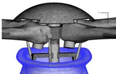
Fig. 7 - Unstructured grid for EC135 main rotor hub
