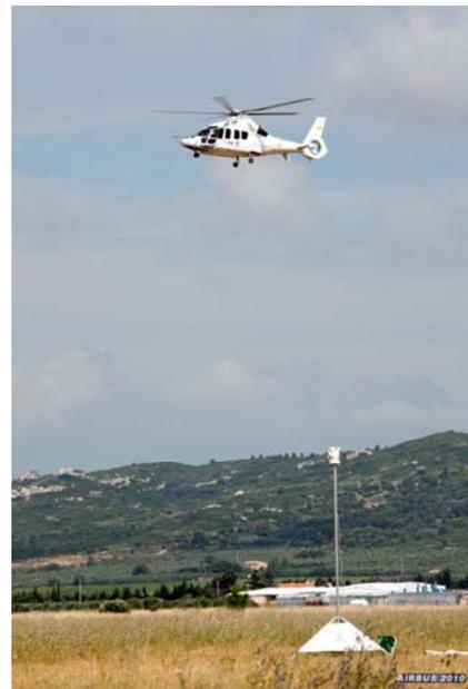
Fig. 14 - EC155 Flight Test for Noise Measurement
