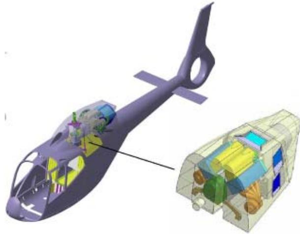
Fig.11- Preliminary demonstrator engine EC120 installation layout
