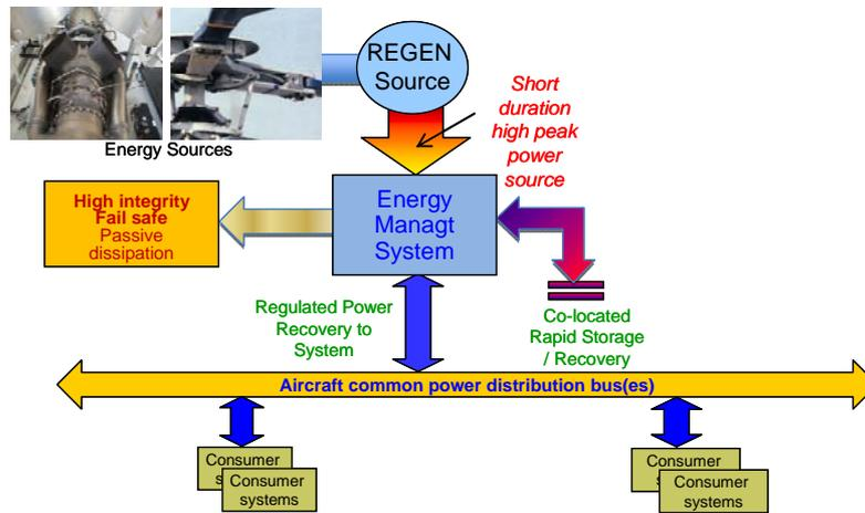
Fig. 9 - Architecture of energy recovery systems
