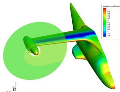
Fig. 8 - ERICA cruise flight CFD computation (CODE-Tilt)
