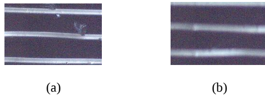
Figure 5: Contrast within frames is used to gauge the focus level
