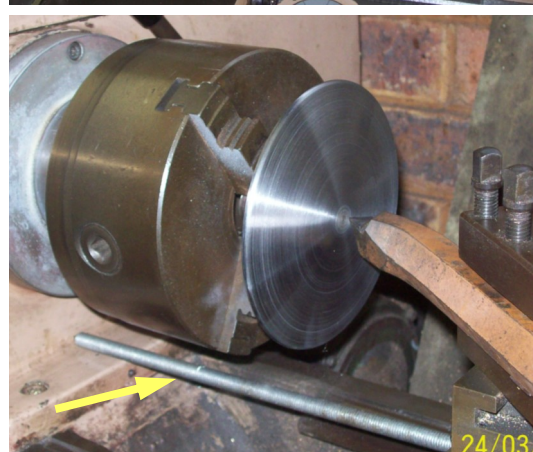
Above: Rays method using the radius bar and large spring. The radius bar is arrowed.
