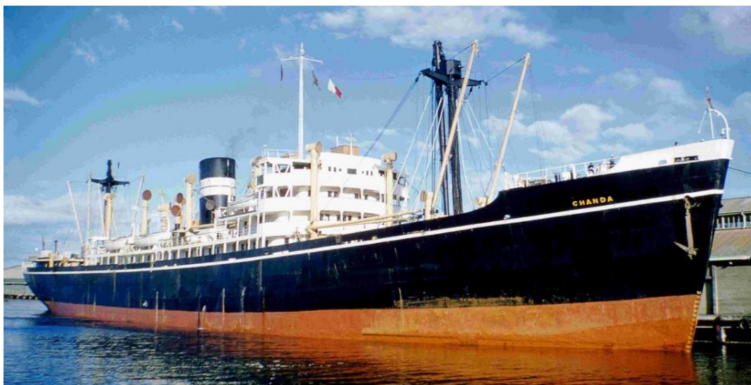
PRECIOUS PEARL as BI's CHANDA at Hobart, 1958/59, wartime rig with signal mast in place of topmasts (unknown/NAA).
