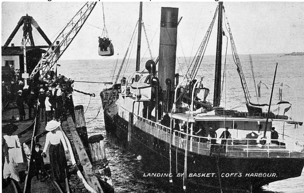
CAVANBA offloading passengers by basket at Coffs Harbour. The swell made alongside disembarkation too dangerous (Flotilla Australia).
