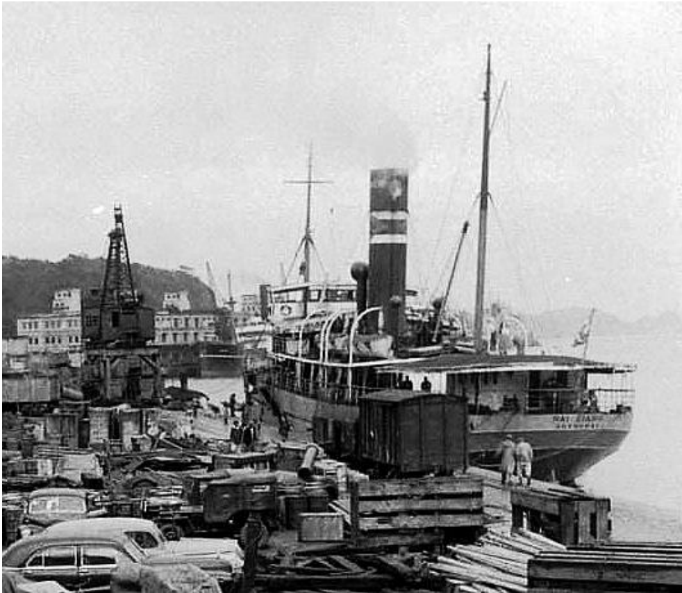
LAI SING at Keelung in mid-1949. As lengthened, LAI HSING carried two boats and had a higher bridge. Also displays the new funnel marking (Attrib. Harrison Forman).
