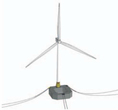
Fig. 3 Typical "Ring Floater" Foundation, and Wind Turbine Generator
