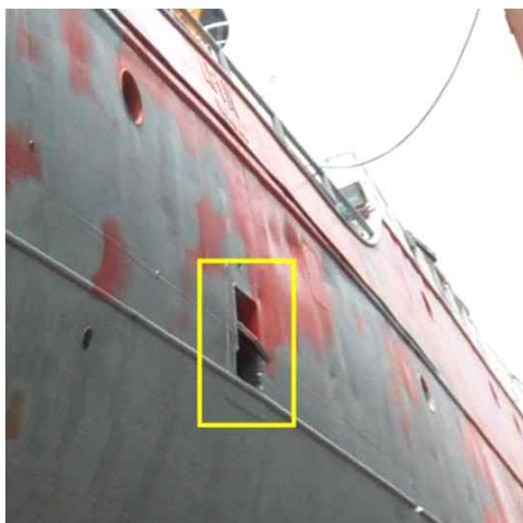
[Image 8] Installation status of sewage discharge outlet of a vessel of same model (right side)
