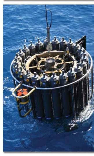
A rosette of filled (24 x 20 litre) water-sampling bottles is hoisted on-board with a steel conducting cable. The orange instrument is an upward looking Acoustic Doppler Profiler (ADCP) that measures current velocities by tracking particle movements in the water. Image: Mike Lucas
