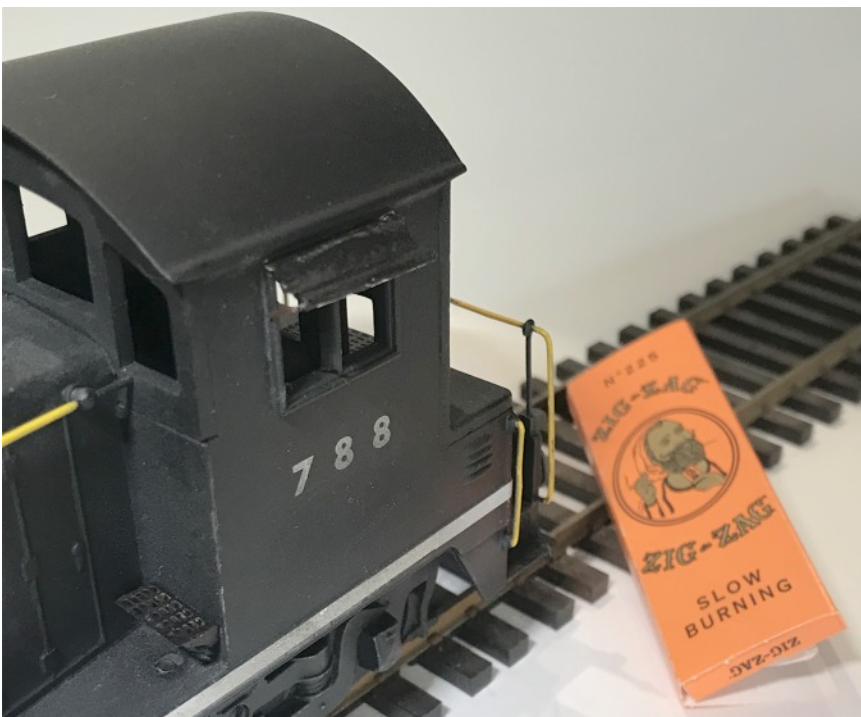
Middle: Under-mounted side air tanks removed and milled flat. Kadee 746 coupler boxes installed. The coupler installation first required removing the pilot to position the shank through the pilot, then assembling the coupler, springs, and box. The pilot with the coupler is then reattached to the body and the coupler box screwed to the body.
