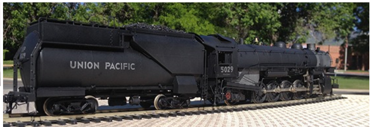
U.P. 5029 is a U.S. Hobbies 2-10-2 I upgraded with a ton of PSC parts. I scratch built the grip box and the water tank extension, and cut in the cab new roof hatches.
