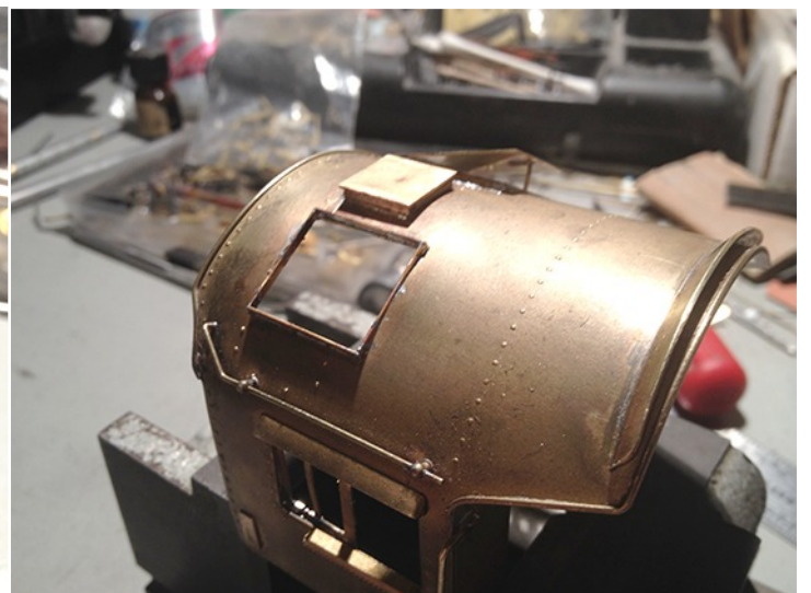
U.P. 5029 is a U.S. Hobbies 2-10-2 I upgraded with a ton of PSC parts. I scratch built the grip box and the water tank extension, and cut in the cab new roof hatches.
