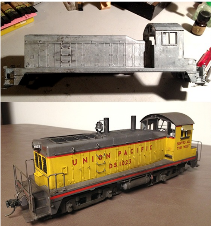
U.P. 1023 is an All Nation NW2 that I did major modifications to. I used KV Models for the stairwells and switching steps. It has CLW sideframes.
