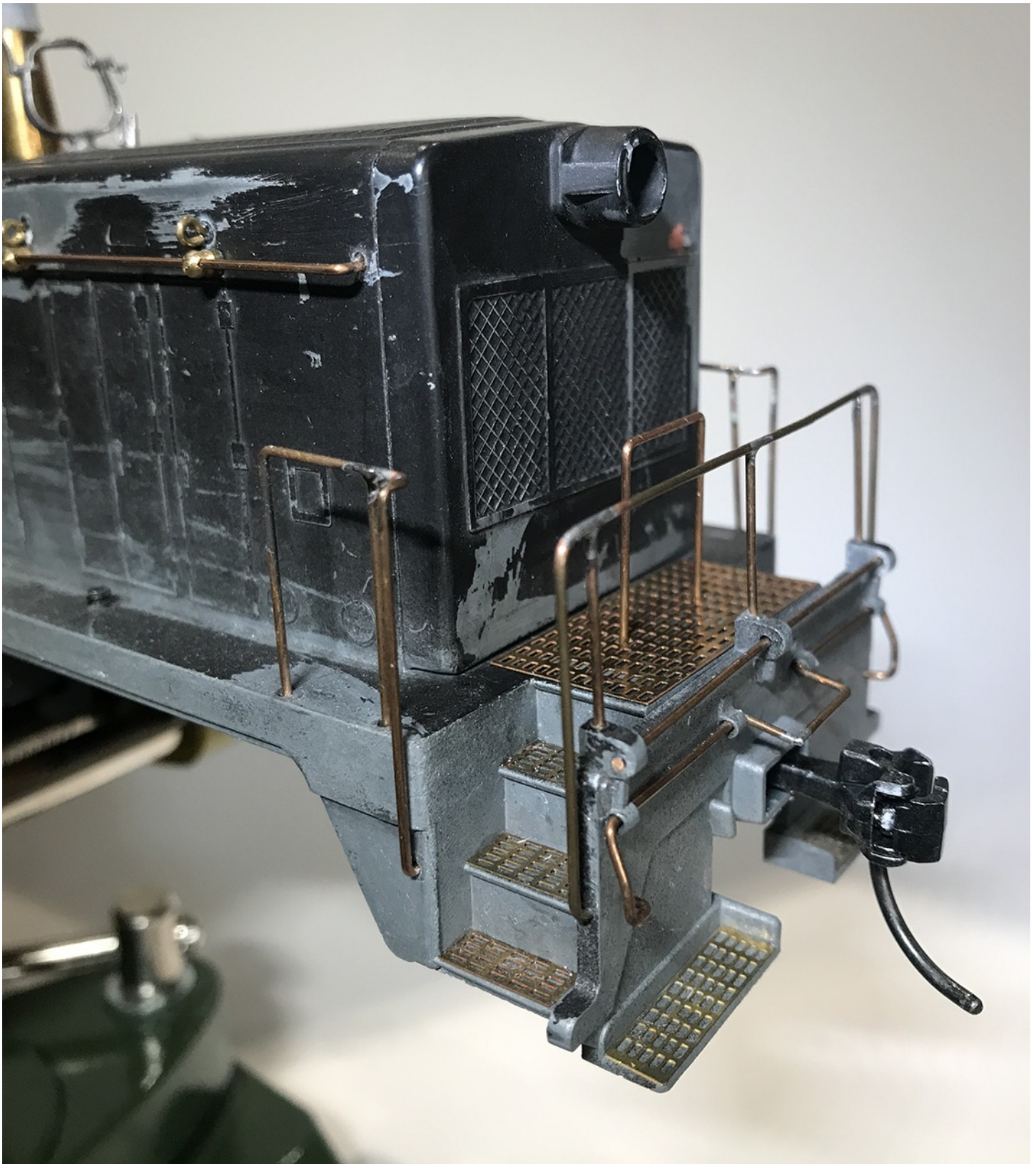
Front railings with coupler and grate detail. The horizontal rods required an extra long drill bit for making holes in the pilot. The rectangular coupler opening required some filing to allow installing the long Kadee 746 coupler shank.
