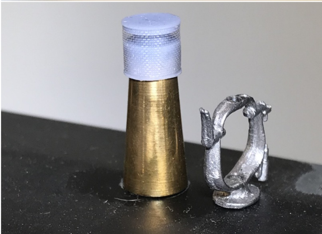
High resolution 3D printed spark arrestor with mesh screen from a resin filter. The finished part was stained with India ink to preserve the mesh openings - avoiding paint that could clog the mesh detail.
