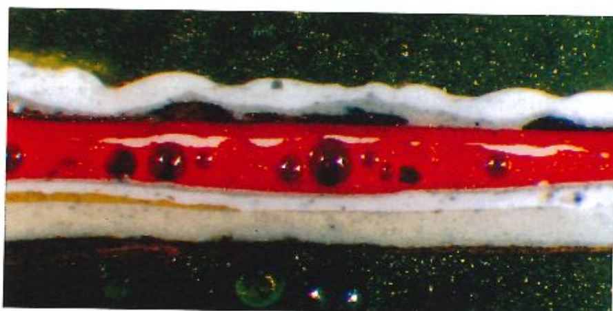
Figure 12.20 Cross-section of the paint sample from the visor lug for the bottom lock.
