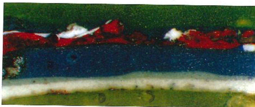
Figure 12.19 Cross-section of a paint sample from the forepeak deck starboard lug.
