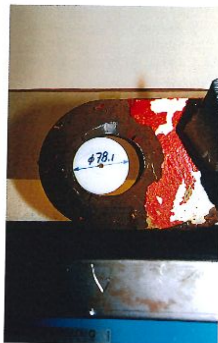
Figure 12.17 The visor lug for the bottom lock with a disc of the same diameter as the bolt inserted.
