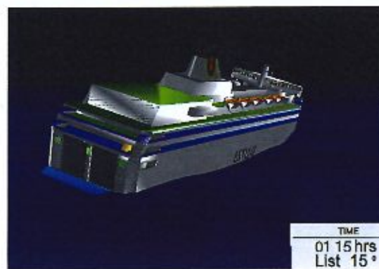
Figure 13.3 Computer-generated pictures illustrating the development of the list and sinking of the vessel. Approximate times, and list in degrees, are shown at bottom right of each picture.
