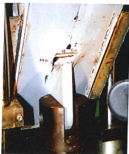
Figure 12.21 Full-scale mock-up test of the side locking lug structure.
