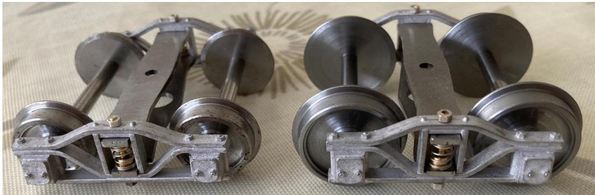
The bogies have suspension in the form of coil springs which are held in place by a 1.6 die brass rod. The example on the Brandbright stand had the rods falling out despite being glued. Luckily there was sufficient length in the brass rod supplied to cut a 10BA thread at each end and thus hold the rods in place with a pair of nuts - hardly prototypical but secure! Above are the Brandbright bogies assembled, 20mm diameter wheels to the left, 25mm to the right. Below is a drawing of same.
