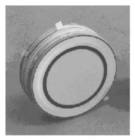
Open Microchannel Plate Imaging Detectors have a design similar to MCP detectors with Metal Anode. Instead of simple metal anode an aluminized phosphor screen is used as a readout device. An electron cloud is drawn across a 0.7 mm gap by a high voltage onto micro-crystalline phosphor screen where the kinetic energy of the electrons is released as light.
