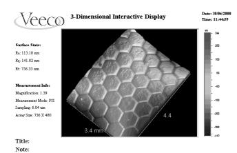
Honeycomb structure of Microchannel Plates. For additional images of Microchannel Plate surface at different spatial resolution <u>click here.</u>
