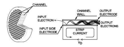
Since the individual channels confine the pulse, the spatial pattern of electron pulses at the rear of the plate preserve the pattern (image) particles incident on the front surface. The output signals are typically collected in any of several ways, including metal or multimetal anodes, resistive anode (one- or two- dimensional), wedge and strip anode, Delay-Line Readout or on a phosphor screen deposited on a fiberoptic or other substrate.
