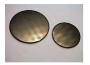
The microchannel plate is an open multiplier intended for registration of particles and radiations. MCPs represent 0.4-3.0 mm thick plates of round or rectangular shape. They have a honeycomb structure and contain in one square centimeter up to one million of separate channels of 5-15  $\mu$  m diameter. In addition to design simplicity, small dimension and absence of external voltage divider, MCPs feature high time and spatial resolution capability.
