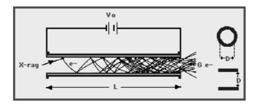
The front plate of a chevron pair for use in X-ray astronomy usually has channels perpendicular to its front surface, since the X-rays emerging from a grazing incidence telescope do so along the surface of a cone. The channels of the rear plate are then at an angle of about 15 degrees. This
