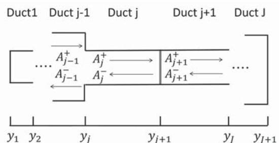
Fig. 3 Quasi-1D model of a generic combustor.
