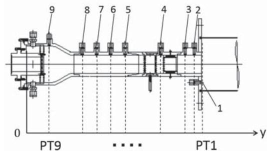
Fig. 2 Mounting positions of the pressure transducers(PT1-PT9).
