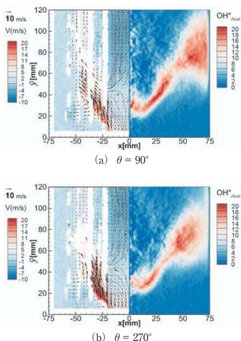
Fig.A1 Phase-resolved velocity field (left) and OH\* in-intensity distribution (right) ( $v = 12.5$  m/s,  $\phi = 0.69$ ). Up-per and lower figures are at  $\theta = 90^\circ$  and  $\theta = 270^\circ$ , respectively. The rectangular blank regions on the velocity maps are the erroneous regions due to the laser sheet reflections on the glass tube surface.
