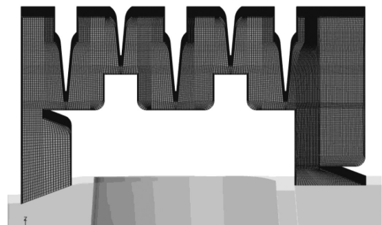
Fig. 6 Computational grid for a shroud leakage flow passage
