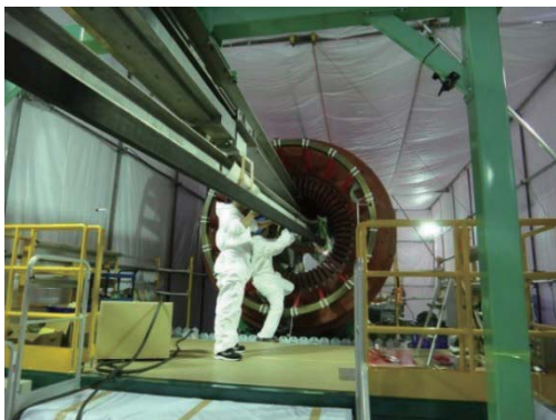
Fig. 14 Stator coil assembly by hanging tool
