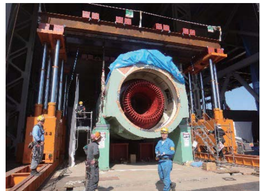
Fig. 16 Stator frame assembly by PJS
