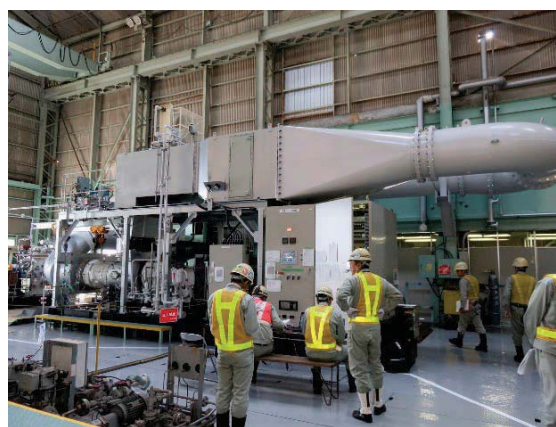
Fig. 9 SB5N in house test facility
