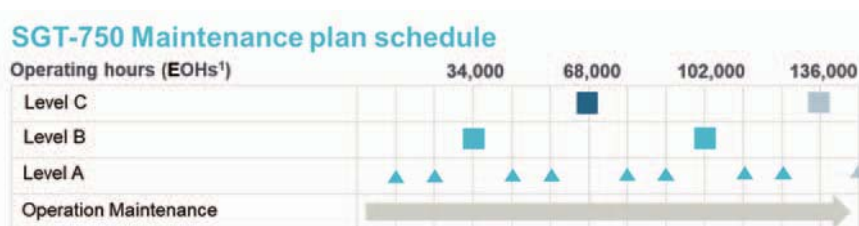
Fig. 9 SGT-750 Maintenance plan schedule (typical)
