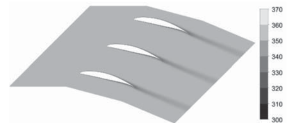
Fig. 6 Total Temperature Distribution past Airfoil Heat Exchangers with k_{\text{solid}} of 202 W/(m·K) in a Main Flow with Constant Total Temperature
