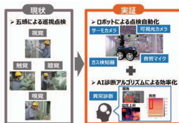
Fig. 5 Automatic inspection by robot
