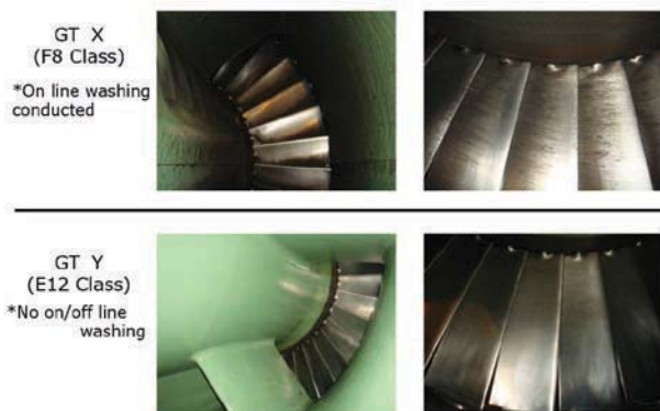
Fig. 4 Comparison photos of IGV
