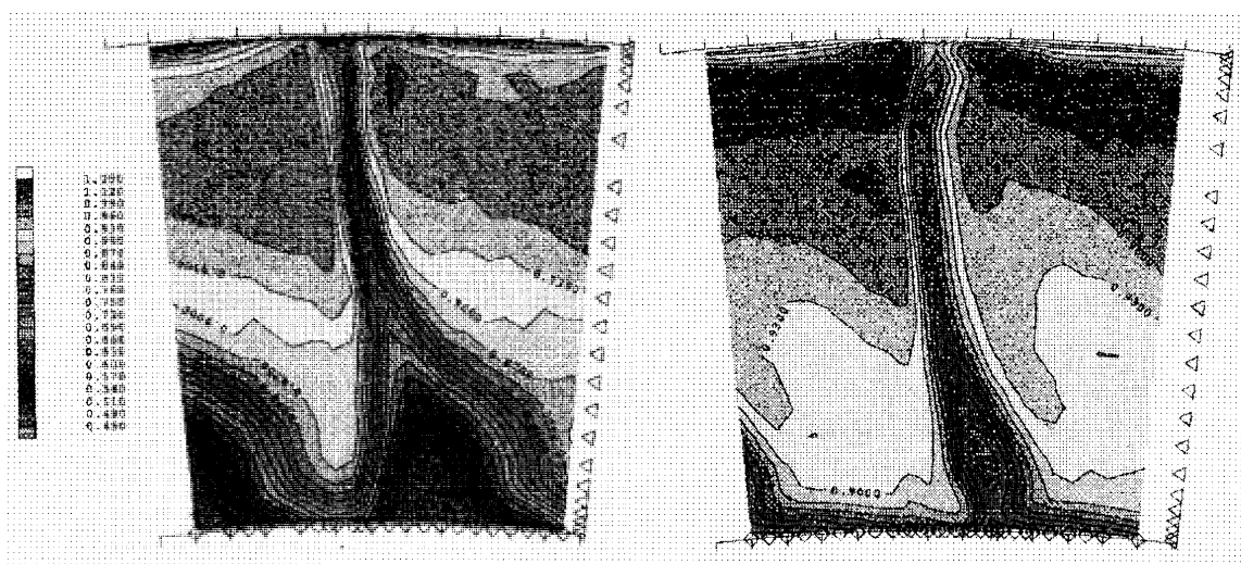
Fig.2 Contours of stagnation pressure coefficient at stator exit for the same rotor and equal flow coefficients
