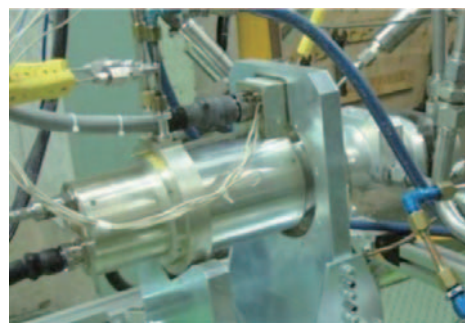
Fig. 8 The electric motor-driven fuel pump with a two channel redundant motor
