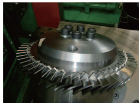
Fig.13 Demonstrator blisk manufactured by LFW (1) .
