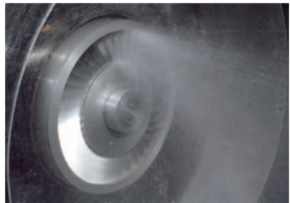
Fig. 5 Two-Phase Impulse Turbine Operating with Single Two-Phase Nozzle
