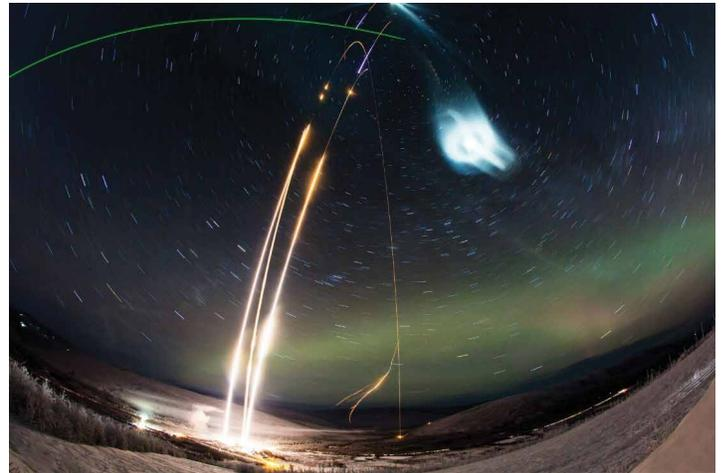
Composite time-lapse photograph of the three Super Soaker rockets launched from the Poker Flat Rocket Range in Alaska on January 26, 2018. The green line in the upper right is the Rayleigh lidar beam. The bright white feature is part of the TMA tracer trail.
