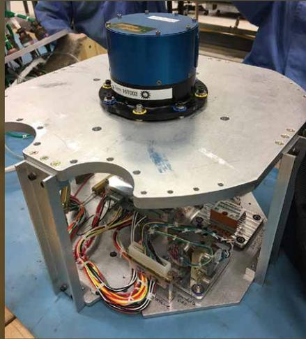
The NSROC developed Tern INS was flown operationally for the first time on 46.021 UO in 2018. The system is designed to generate high quality, reliable body rate and acceleration measurements, attitude propagation, and navigation solutions.
