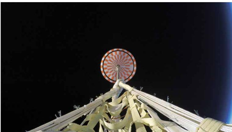
ASPIRE SR03 in flight after deployment from sounding rocket.
