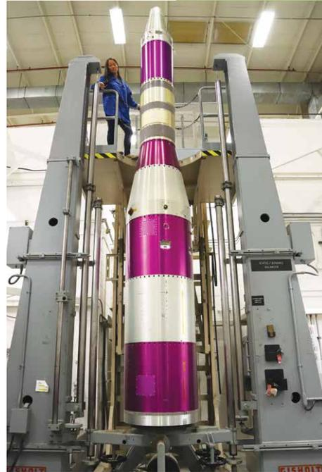
NSROC Testing and Evaluation Lab intern with an ASPIRE payload on the balancing table.
