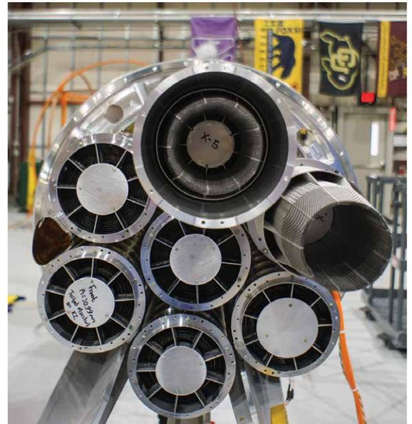
Front view of the 7 FOXSI-3 optics modules. Note the addition of collimators in front of two modules. These collimators are 3D printed with a fine honeycomb structure to block stray light.
