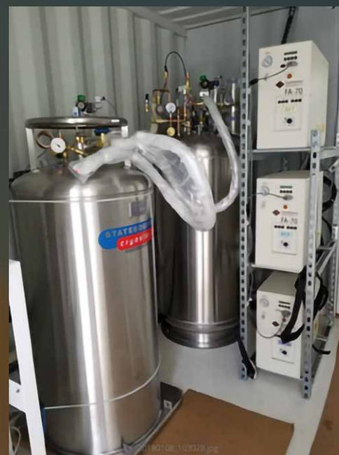
Several next generation instruments and detectors require significant LN2 for cooling prior to launch. In many of the remote launch areas, supply chain logistics makes delivery difficult, expensive, or impractical. To facilitate payload cooling requirements, SRPO invested in a mobile LN2 plant.
