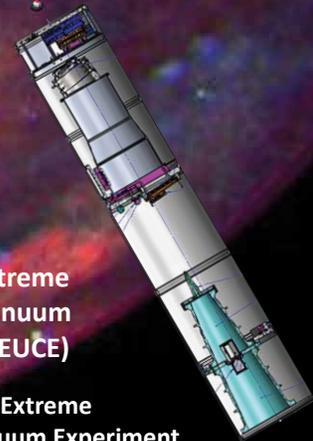
The Dual-channel Extreme Ultraviolet Continuum Experiment (DEUCE) is a spectrograph operating from 650 – 1100Å. DEUCE is designed to measure how much ionizing photons B stars, such as the target star for the 2018 mission  $\beta$  Canis Major, produce.
