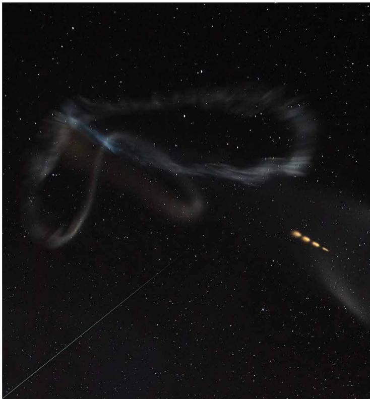
Super Soaker TMA tracer trail and the Rayleigh lidar beam.
