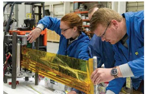
**University of Nebraska - Lincoln:** Partnering with NASA's Langley Research Center in Hampton, Virginia, the team tested a deployable and retractable boom and solar blanket for space applications, including sounding rockets, CubeSats and small satellites.
