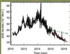
SDO EVE measurement of the He I 584 Å emission is shown in black. The calibration rocket flights are shown as green squares, and the trend between the last calibration in 2016 to this new one in 2018 provides the correct trend for solar cycle variability.
