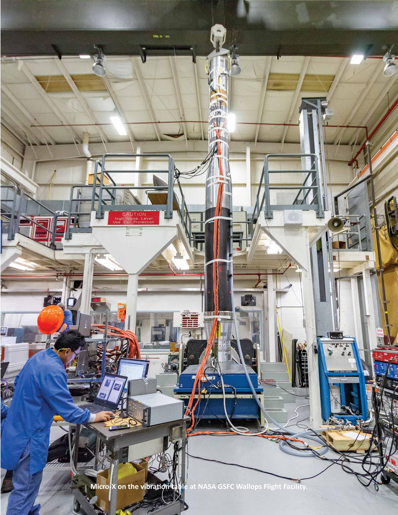
Micro-X on the vibration table at NASA GSFC Wallops Flight Facility.
