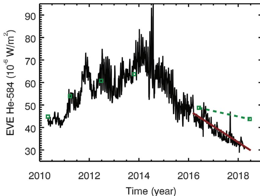
SDO EVE measurement of the He 584 Å emission is shown in black. The calibration rocket flights are shown as green squares, and the trend between the last calibration in 2016 to this new one in 2018 provides the correct trend for solar cycle variability.
