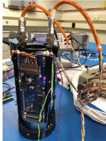
Sub-payload control card bench testing
