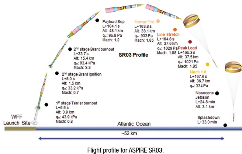
Three flights, using two-stage Terrier-Black Brant vehicles, were conducted during FY 2018. The parachute inflation loads were increased successively, starting with 35,000 lbf and ending with nearly 70,000 lbf.
