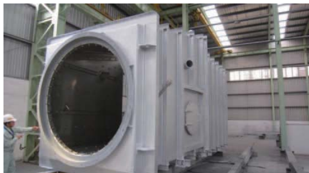
Fig. 17 Sample of Exhaust duct
