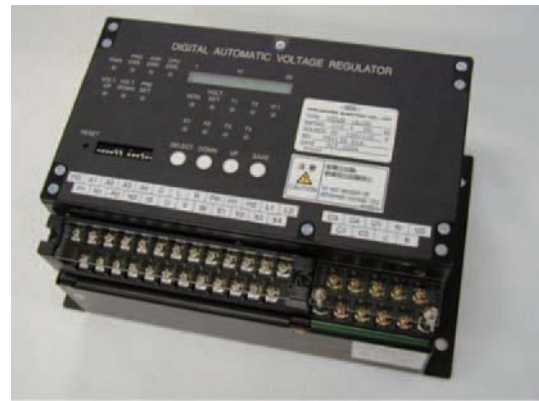
Fig. 14 Automatic voltage regulator
