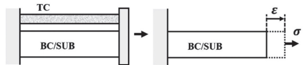
Fig. 4 Mechanistic model for TBC system
