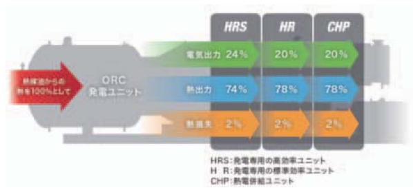
Fig. 9 Heat balance of ORC unit
