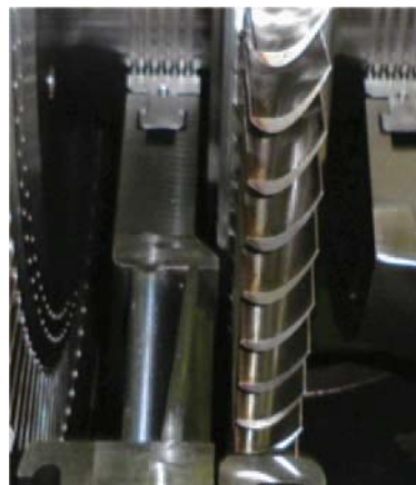
Fig. 6 Last stage including laser-quenched rotating blades
