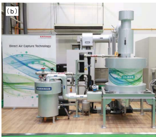
Fig. 7 (a) Proof-of-concept test equipment (0.5 kg/d) (b) lab-scale demonstration equipment (5 kg/d)
