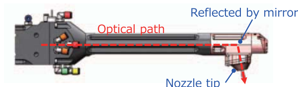
Fig. 16 LMD nozzle for inner surface cladding
