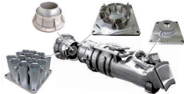
Fig. 13 Combustor rapid prototyping by AM
