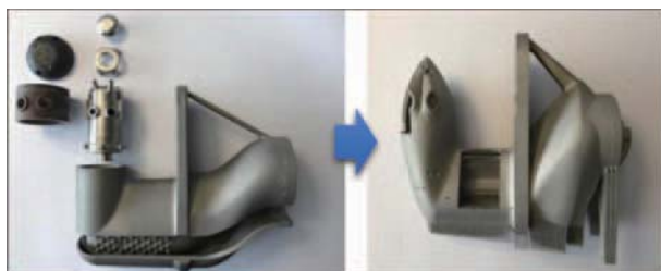
Fig. 6 GT26 lance injector demonstrating assembly reduction.
