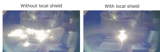
Fig. 5 Differences during Ti-6Al-4V printing with and without local shield
