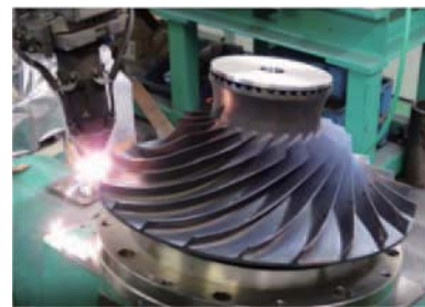
Fig. 11 Repairing of impeller by LMD
