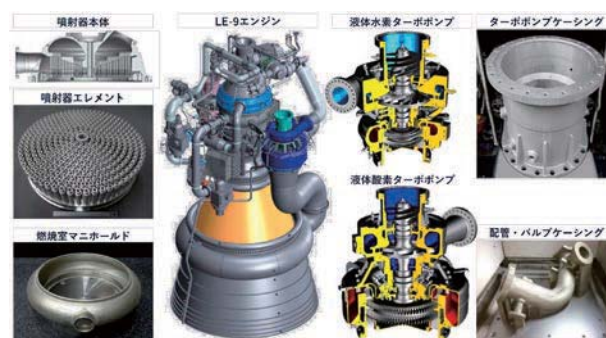
Fig. 12 Critical components of LE-9 using additive manufacturing technology
