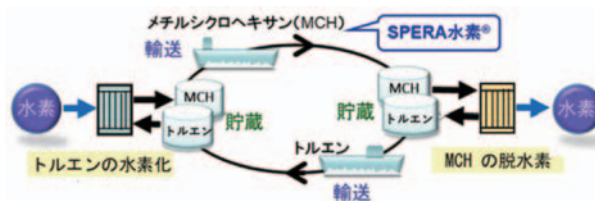
Fig. 1 Scheme of SPERA hydrogen system
