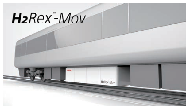
Fig. 8 Image of H2Rex™-Mov module installed on a railroad
