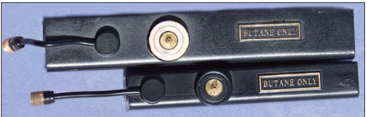
Photo 1 - Fuel Tank Comparison. Top: Original – Bottom: Accucraft replacement
