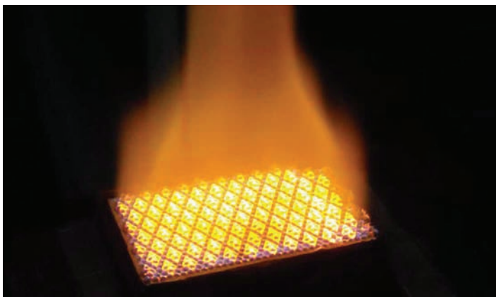
Photo 11: The burner is tested on the bench.
