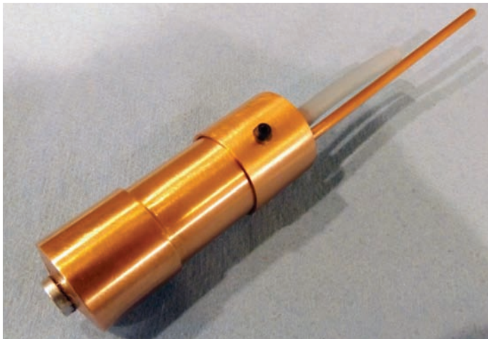
Assembled catch can: Magnet holds it in place.
