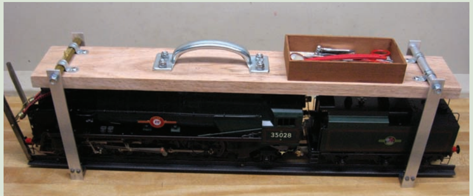
Carrier filled: Complete with small parts box on top of the board.
