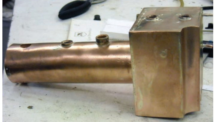
Photo 8: Finished boiler has a recess for lubricator.
