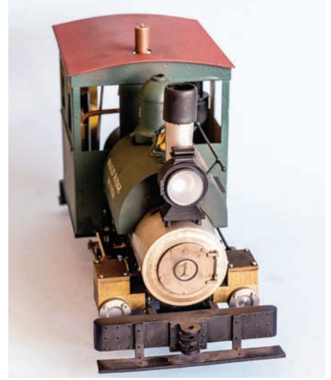
Author's alterations: New paint and the new smoke stack, which has a tube inside to catch 'spooce.'
