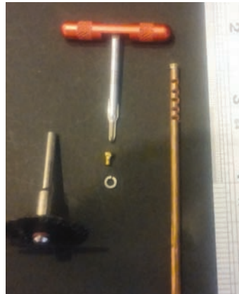
Exhaust mod: Rosenblum added a screw and cut slots in the pipe.
