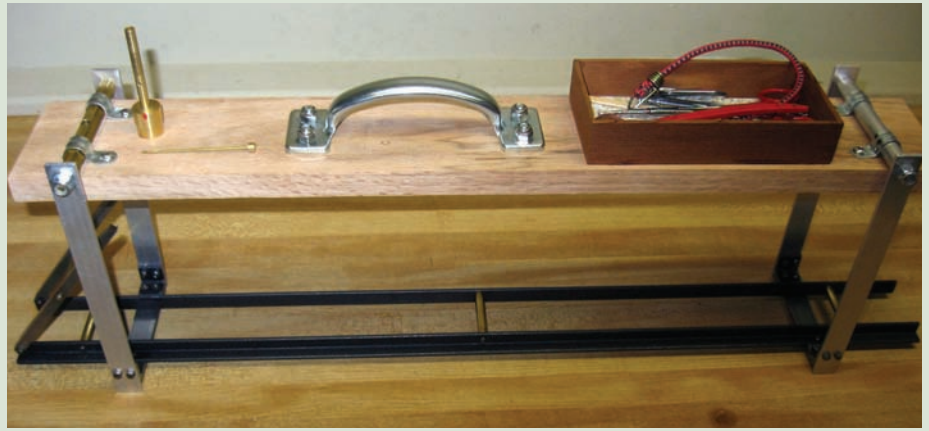
Carrier: Constructed of angle metal and oak, with a sturdy handle.
