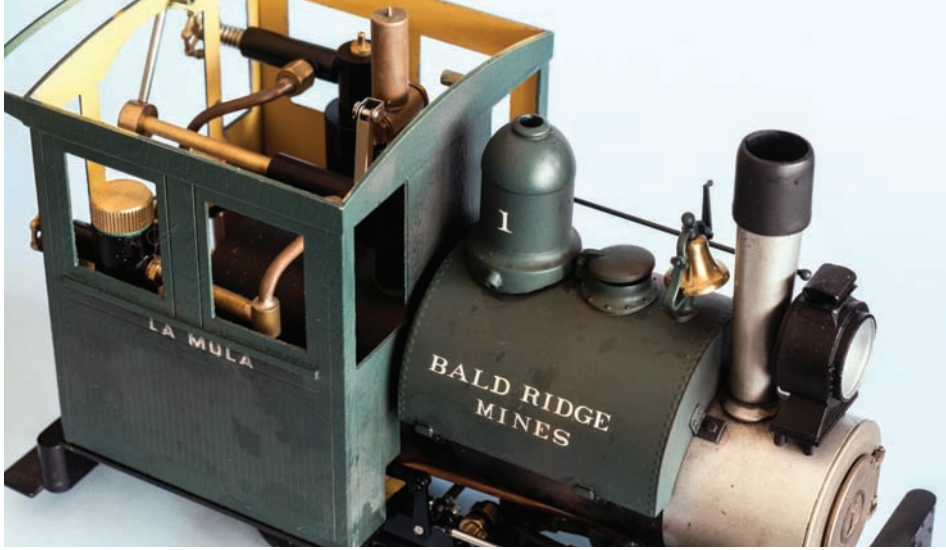
Author's alterations: New paint and the new smoke stack, which has a tube inside to catch 'spooce.'
