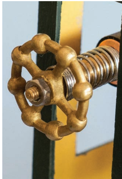
Cast brass: Wheel to control gas protrudes slightly out of the window for easy handling.
