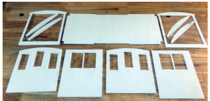
Styriene: Walls and roof pieces are cut out.
