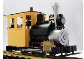
1:20.3-scale, Gauge 1 (45mm) butane fired
