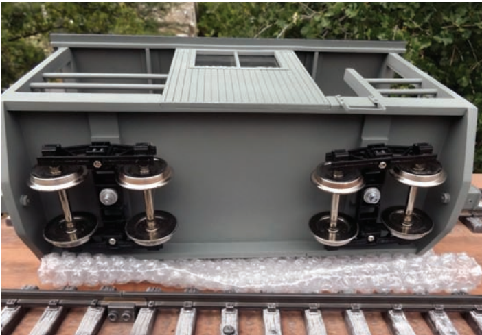
Wheels: Commercial trucks attached to underside.
