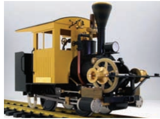
1:20.3-scale, Gauge 1 (45mm) butane fired
