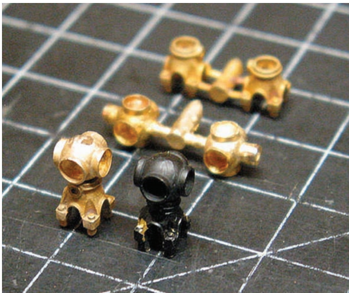
Lost wax: Castings by Triple R Services of an Aster PRR K4 Marker light (original on right in black).
