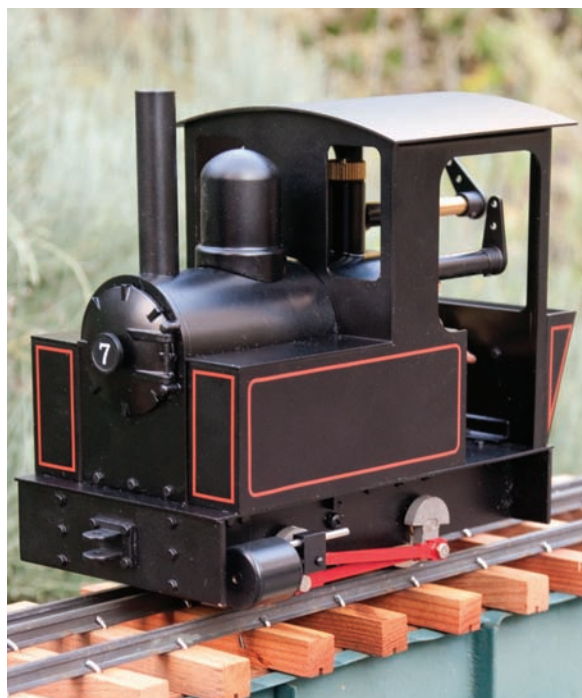
Outside action: Adding dummy cylinders to your Accucraft 'Dora' makes the engine look much more locomotive-like. This project involves some basic machining.
