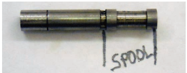
Photo 1: ‘Ruby’ valve piston showing spool portion.
