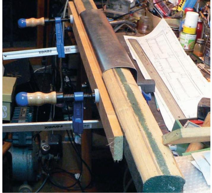
**Two more bends:** *Left, the quarter-round in place, a second bend is put into the roof. Right, the full form for the roof's big curve is placed into the vise, allowing for the top of the roof to be formed.*
