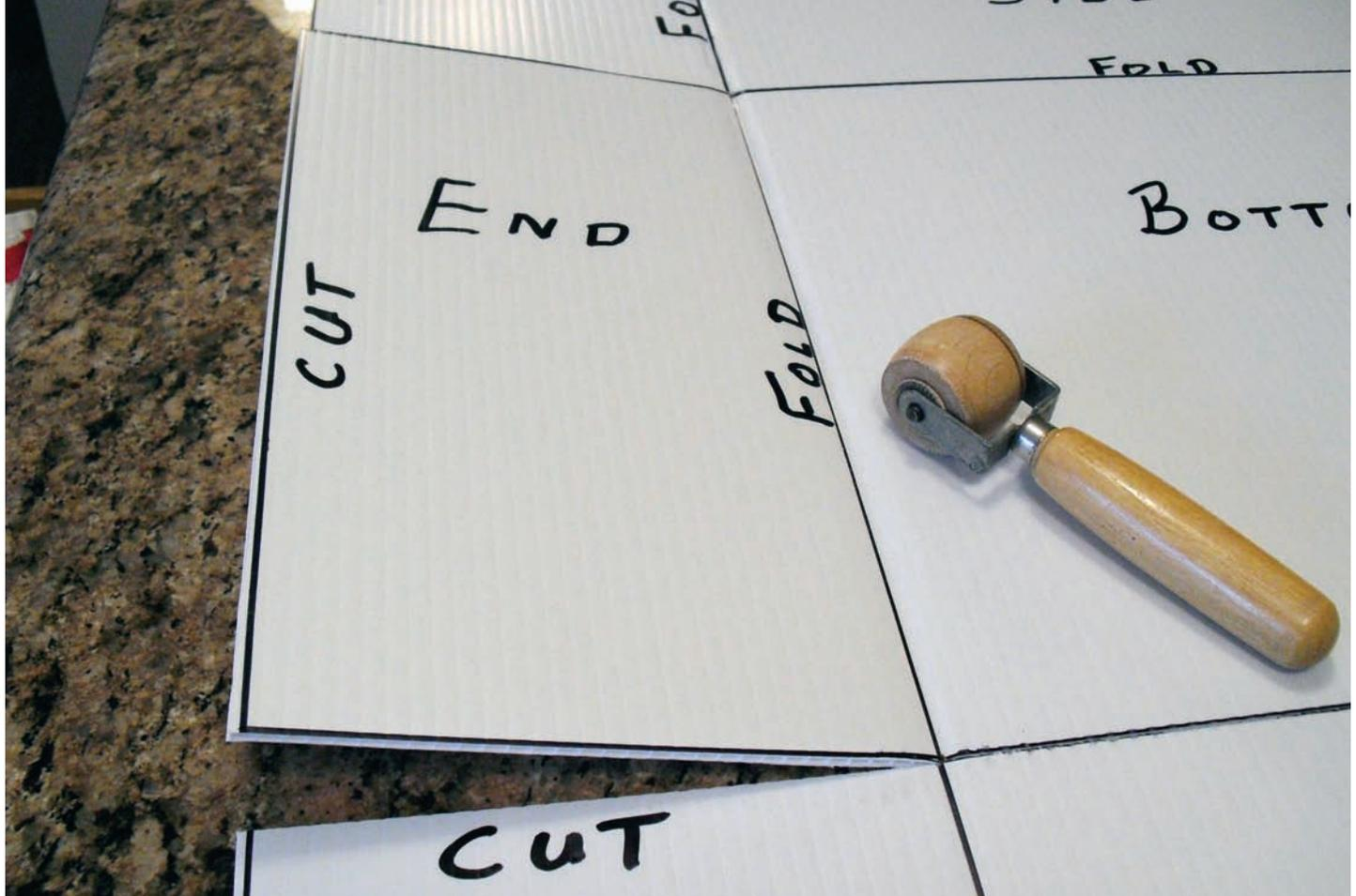
**First cut:** After cutting the corrugated plastic, use the wallpaper seam roller to compress at folding points.
