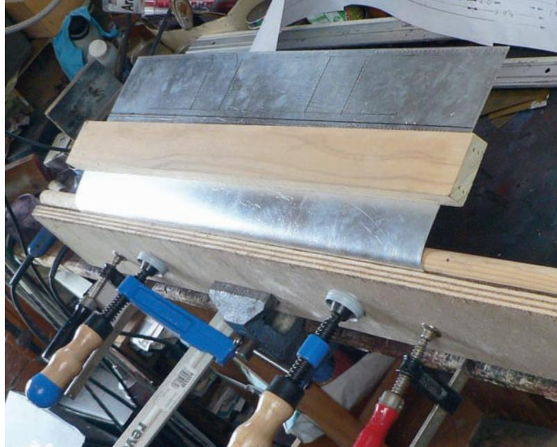
**Vise and clamps:** A first attempt at making a bend in the aluminum (where a half-round piece of wood was used; later a quarter-round was substituted). The vise holds the work to the bench.
