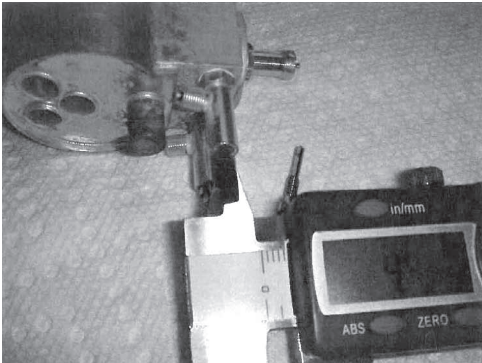
Photo 3 - Measuring the valve body ID.
