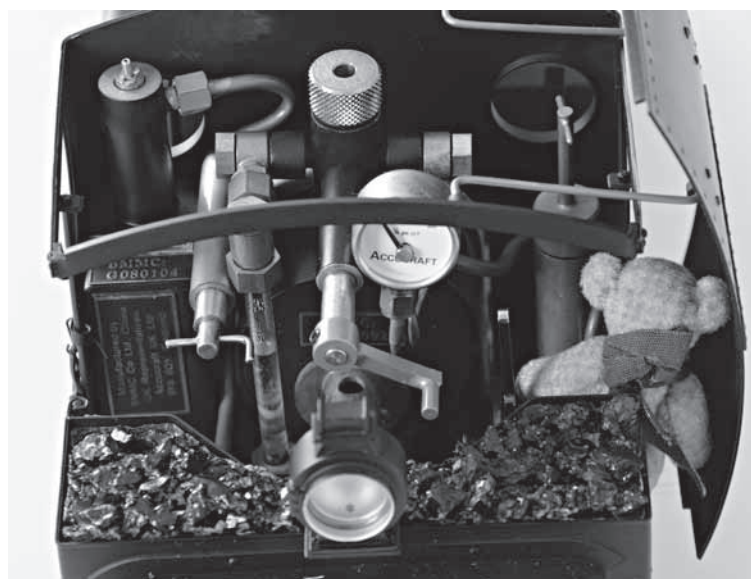
The coal load is self made. There is space enough for batteries and a servo if needed beneath it. (We prefer to run by hand)
