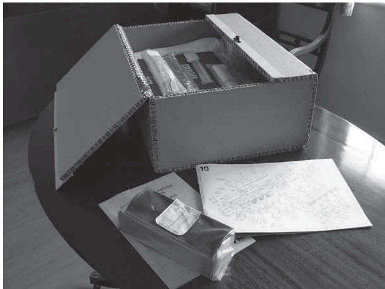
The Aster A3 Kit. All kits come boxed in extremely tough containers. In these are smaller boxes in which are housed all parts wrapped and sealed. Also included are the instruction manual and book of isometric drawings, sealant, tools, etc.
